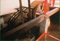
Main shaft of a spinning mill
