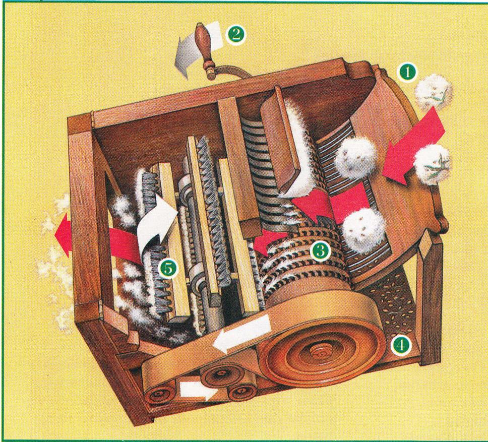
① Cotton bolls, made up of fiber and seeds, are fed into the cotton gin. The red arrows show the path of the cotton through the gin.
