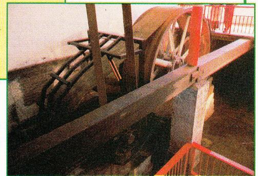
Main shaft of a spinning mill
